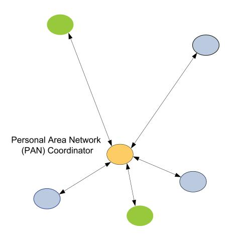
Digi's XBee<sup>TM</sup> 802.15.4 OEM RF modules can be set up to operate in a point-to-point, point-to-multipoint or a peer-to-peer configuration. While standard 802.15.4 always requires a coordinator, the Digi radios are set up so that a coordinator is not required.
