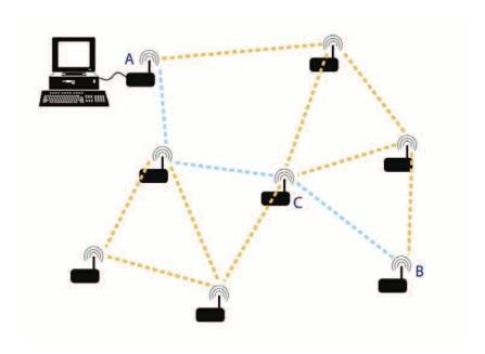
As an example, in the figure above suppose you want to transmit data from point A to point B, but the distance was too great between the points. The message could be transmitted through point C and a few other radios to reach the destination.
